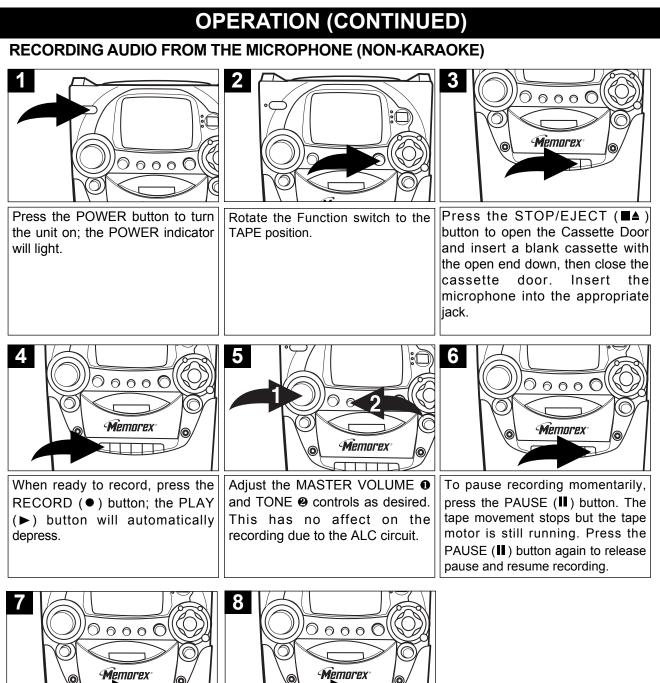
To stop recording before the tape ends, press the STOP/EJECT (■▲) button. The PLAY (►) and RECORD (●) buttons are released and the tape motor shuts off.
